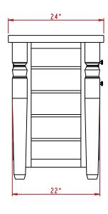
This furniture style island is manufactured using the highest quality furniture grade hardwoods and MDF. The island features two working drawers and an open cabinet with adjustable shelf on one side and a decorative panel on the reverse side with fully adjustable shelves on both ends. The drawers are dovetailed solid hardwood and are mounted on full extension undermount soft-close slides. Cabinet features integrated soft-close hinges. Available in Aged Black or French White finish.
